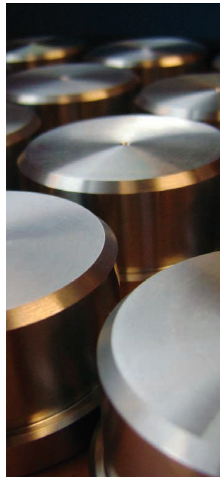
We use these machined stainless steel fixtures to align the voice coil and the diaphragm within a hair's width. This level of precision in manufacture insures decades of uninterrupted performance.
